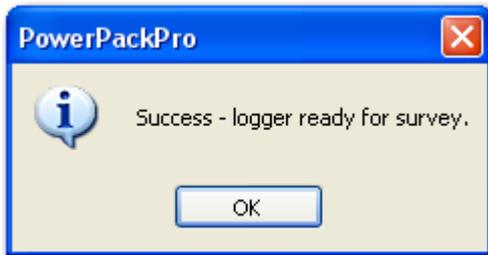
**NOTE:** Setting the logger will synchronise the logger clock to the PC clock time and delete any records in the logger memory.
